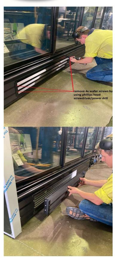
Unscrew the Wafer Screws and Remove the Grille.
