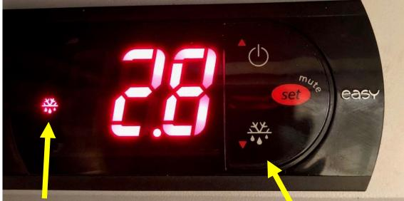
**Defrost Symbol** - when this is showing the case is in defrost mode. To manually start a defrost, press and hold the defrost button for 3 seconds.
